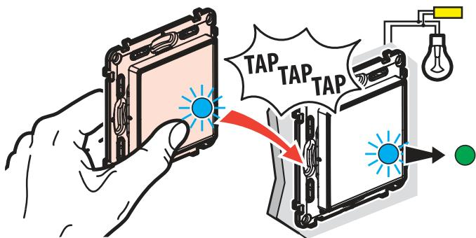
The LEDs of the 2 products flash blue and then light up in solid blue. The wireless control indicator goes off and the connected switch indicator turns green.
