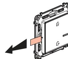
Remove the battery's protective strip to power the wireless general control.
